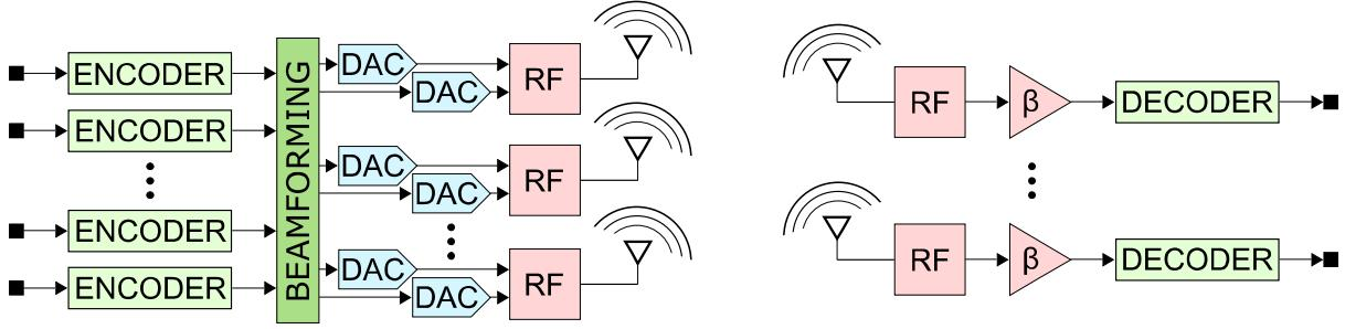
**Fig. 1.** System model of 1-bit beamforming in massive MIMO systems with  $B$  base-station (BS) antennas serving  $U \ll B$  users. The BS (left) is equipped with one 1-bit digital-to-analog converter (DAC) per in-phase and quadrature component. 1-bit beamforming minimizes the power consumption at the BS and mitigates multi-user interference (MUI) at the user side (right).
