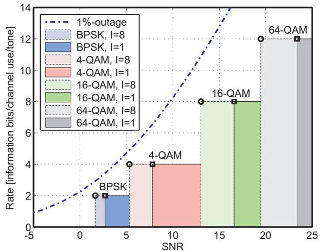
Fig. 11. 1%-outage-capacity compared to the SNR operating points of SISO STS-SD for 1% FER. Squares and circles correspond to SNR operating points realized by  $I = 1$  and  $I = 8$ , respectively.
