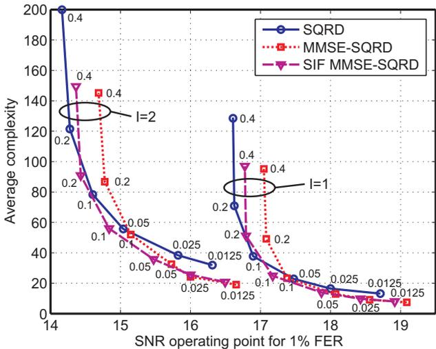
Fig. 4. Performance/complexity tradeoff of SISO STS-SD with SQRD, MMSE-SQRD, and SIF MMSE-SQRD. The numbers next to the curves correspond to normalized LLR clipping parameters.
