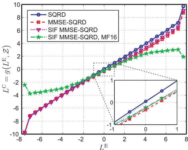
Fig. 6. Different LLR correction functions for  $I = 1$  at SNR = 16 dB with  $\mathcal{Z} = \{L_{\max}, D_{\text{avg}}, \text{SNR}, T\}$ .
