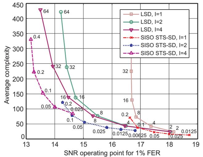
Fig. 5. Performance/complexity tradeoff of LSD [1] and SISO STS-SD, both using SQRD. The numbers next to the curves correspond to the list size for LSD and to normalized LLR clipping parameters for SISO STS-SD.
