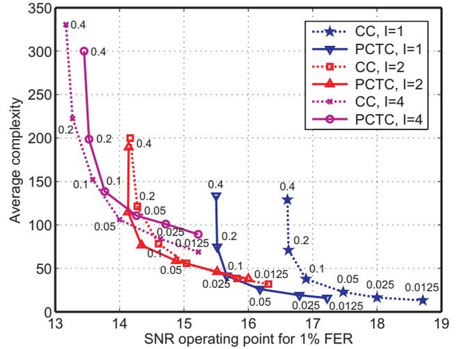
Fig. 8. Performance/complexity tradeoff of SISO STS-SD with SQRD (without regularization) and LLR correction. Comparison between parallel-concatenated turbo codes (PCTCs) and convolutional codes (CCs).
