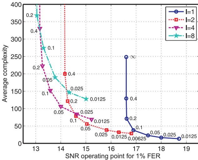
Fig. 3. Performance/complexity tradeoff of SISO STS-SD with SQRD. The numbers next to the curves correspond to normalized LLR clipping parameters.
