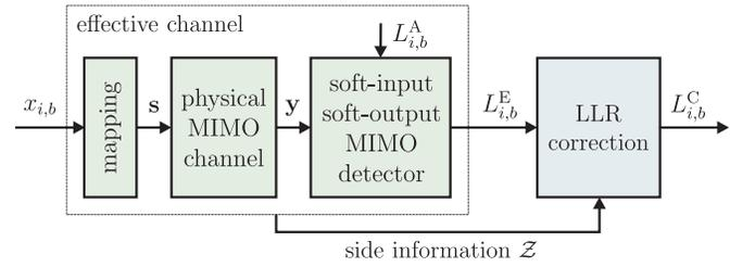
Fig. 2. LLR correction post-processes the LLRs resulting from the effective channel using side information  $\mathcal{Z}$ .
