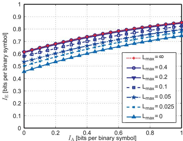
Fig. 9. ITC of SISO STS-SD at SNR = 12 dB for different (normalized) LLR clipping parameters.
