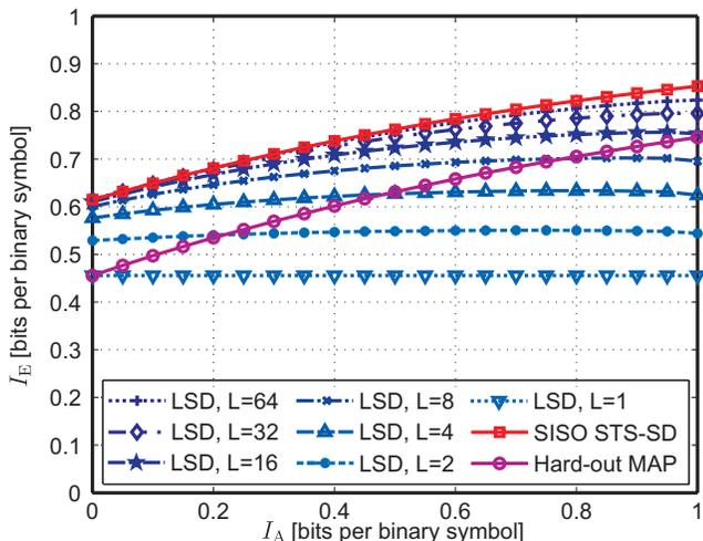
Fig. 10. ITCs of LSD, hard-output MAP (corresponding to  $L_{\max} = 0$ ), and max-log optimal SISO STS-SD (corresponding to  $L_{\max} = \infty$ ) at SNR = 12 dB.
