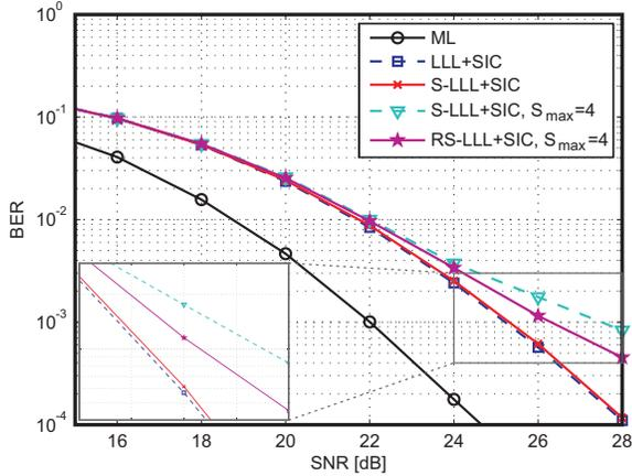
Fig. 1. Uncoded bit error-rate (BER) for LR-aided SIC in an i.i.d. Rayleigh fading  $M_T = M_R = 4$  MIMO system with 16-QAM. Remapping to the finite lattice  $\mathcal{X}$  is done by quantization [11].  $\delta = 0.75$  has been used for the LLL algorithm, while for the Siegel LLL-variants (S-LLL and RS-LLL)  $\epsilon = 0.5$ . ML performance is shown as a reference.
